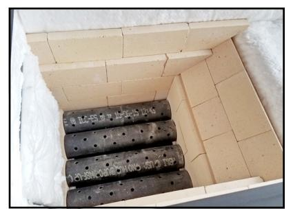
This photo shows brick placement of the side wall and ramp of the firebox. After bricking, remember to then install a second layer of insulation between the top arch rail and the top brick layer. (See Figure D on page 2)
