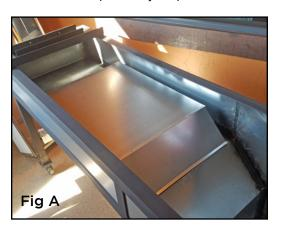
3. Using one long piece of insulation, insulate the rear wall of the arch (by the exhaust), down the arch bed (over the top of the riser if applicable), and into the firebox. This long piece of insulation will end at the firebox's rear brick ledge. No insulation is required below the brick ledge, but some folks do opt to use remaining scraps of insulation on the floor and sidewalls.
