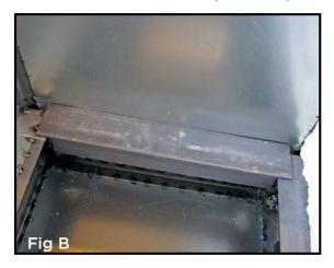
The pieces of angle iron which were provided with the Corsair Arch should be installed on the left and right sides of the firebox to bridge the front and back ledges. This is where the bricks will sit.
