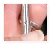
Find the dimple on the stem of your thermometer. This dimple indicates the minimum amount of the stem that must be submerged in order to get the most accurate reading.
