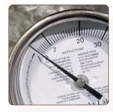
The needle of the thermometer should make one full revolution before coming to rest on the "O". If the needle does not land on zero, use a 6 mm wrench to turn the calibration screw on the back of the thermometer. This will adjust the needle's position. Then re-immerse the stem in the boiling water to check your adjustment.
