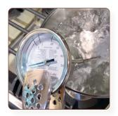
Wear protective gloves and hold the thermometer in the boiling water with a set of tongs, submerging the stem at least up to the dimple mark. Do NOT allow the thermometer's stem tip to rest on the bottom of the pot.
