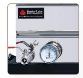
Now that your thermometer has been calibrated, the bold "7" mark will represent finished syrup. Install the thermometer on your evaporator pan using plumbers tape to enhance the seal and prevent thread binding.
