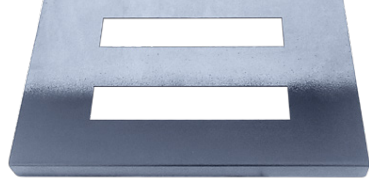
FIG 1D | DAMPER SLIDE: Paint the top and the underside of THIS END ONLY . In contrast, painting the entire length of the Damper may inhibit it from sliding smoothly.
