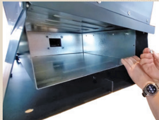
Fig H - Insert the Pressure Cabinet in the Arch
