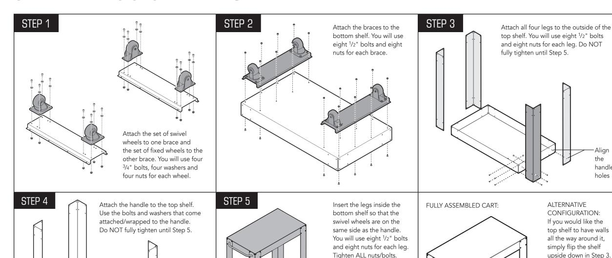
**ALTERNATIVE** CONFIGURATION: If you would like the top shelf to have walls all the way around it, simply flip the shelf upside down in Step 3. The finished cart would then look like this:
